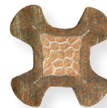
Indenter Crimp Cross-Section Across Axis
